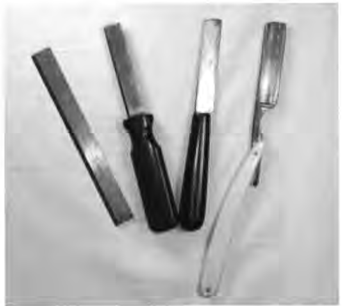
Various reed knives left-to-right: Craftsman single bevel jointer blade, single bevel reed knife, double bevel reed knife, double bevel straight razor from the 1800's
