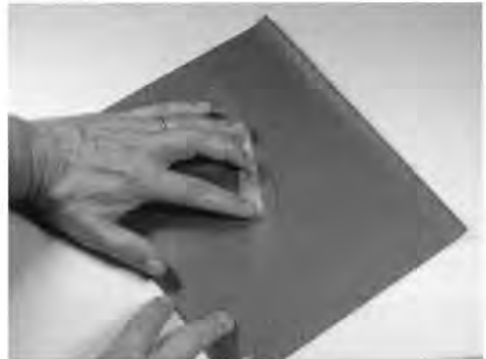
Photo 5 Flattening the reed on sandpaper
