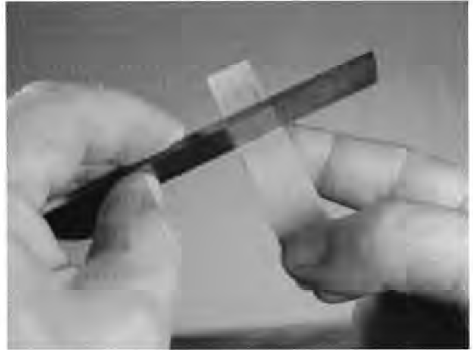
Photo 4 Flattening the back of the reed with a reed knife
